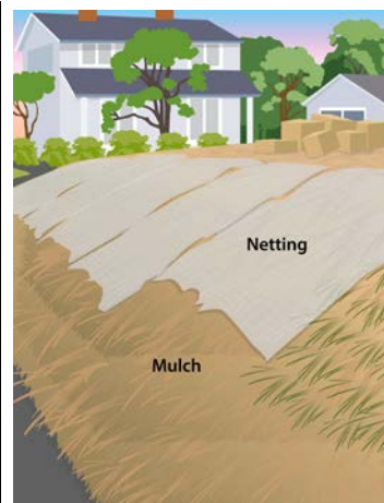
Use wildlife-friendly netting to secure mulch on slopes.
