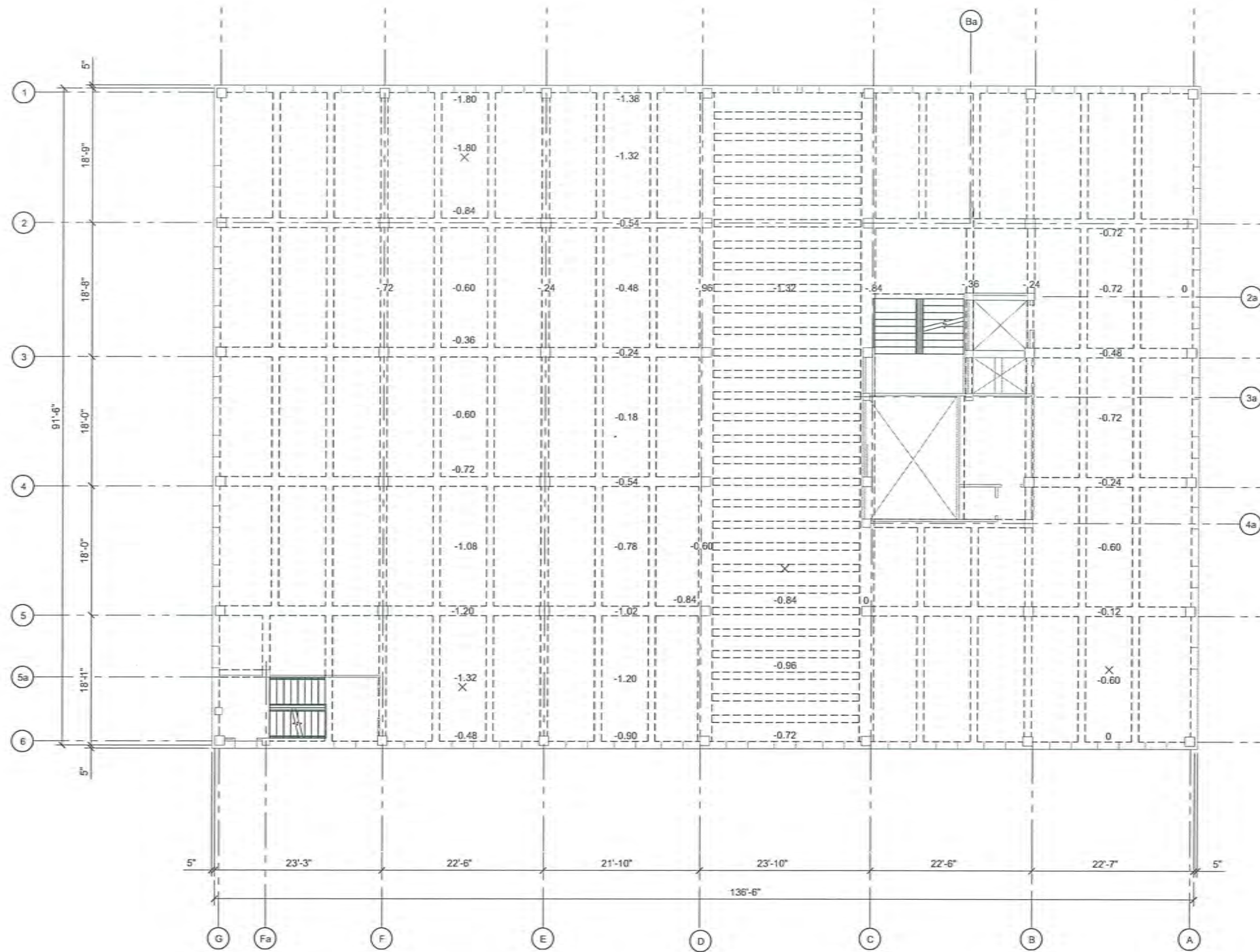
A THIRD FLOOR - PLAN - MEASURED DEFLECTIONS
